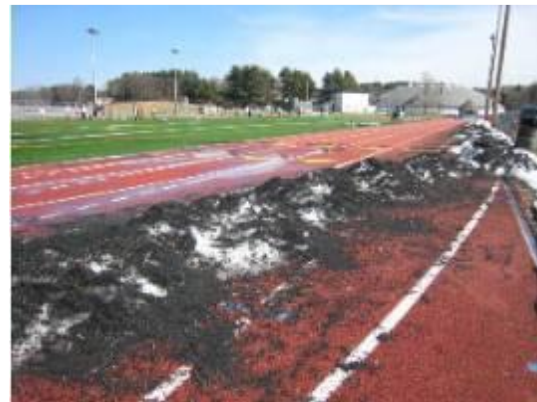
Figure 14 - Photo: Degraded Crumb Rubber
